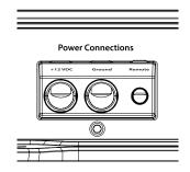
The amplifier's "+12 VDC" and "Ground" connections are designed to accept up to 4 AWG copper power wire.
