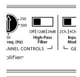
1) "High-Pass Filter" Controls (Front and Rear channels) or "Low-Pass Filter" Control (Sub Channel): These switches allow you to select filter slopes or defeat the filter(s) completely.
