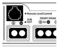
When connected to the amplifier, the HD-RLC operates as follows. At full counter-clockwise rotation, the audio will mute completely. At full clockwise rotation the level will be the same as if the HD-RLC was not connected at all. In other words, it operates strictly as a level attenuator.
