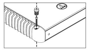
The standard method of mounting requires removal of the four corner caps with the 4 mm hex wrench included with your amplifier. Using appropriate mounting screws (not included), secure the amplifier in all four corners and replace the corner caps to cover the screws.
