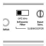
With ported enclosures, the use of the "Infrasonic Filter" is highly recommended to protect the speaker(s) from excessive excursion below box tuning.
