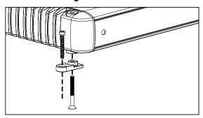
Lateral Mounting Feet are also included with your HD900/5 to provide an alternative mounting option. Each mounting foot should be attached to the bottom of the amplifier by screwing the provided bolt into the bottom of the amplifier and up into the corner cap with the supplied 2.5 mm hex wrench. Next, using appropriate mounting screws (not included), secure the amplifier by its four Lateral Mounting Feet.
