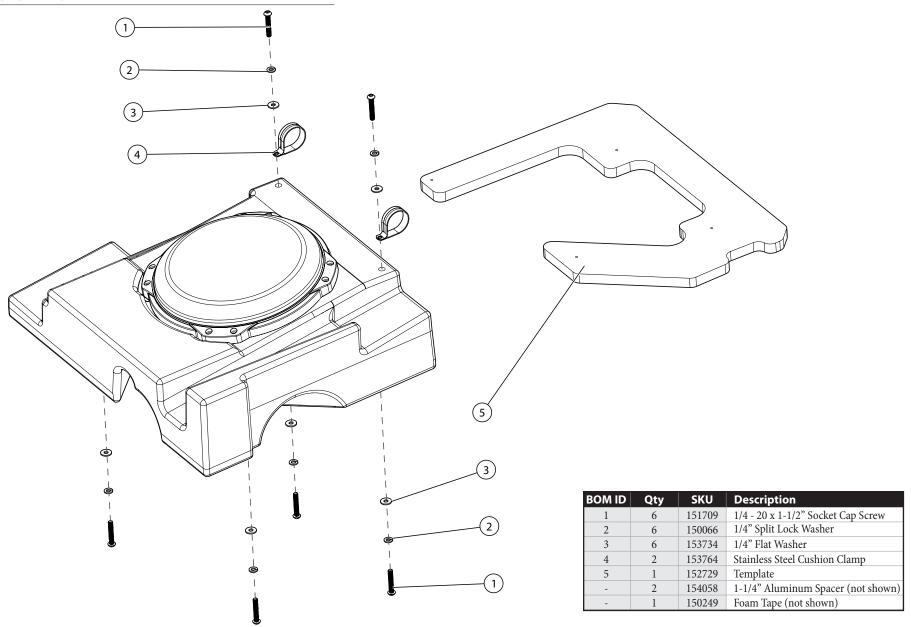
Note: For optimum performance, JL Audio recommends applying the included Foam Strips (or sound damping material) to surrounding plastic panels to reduce unwanted vibrations.
