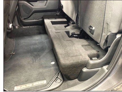
STEP 6 Place the Stealthbox® into the vehicle. Center the enclosure, and align the two upper slots in the Bracket with the factory inner seat bracket bolt holes.
