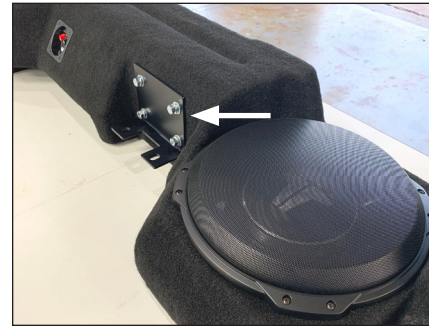
STEP 5 Place the enclosure on a flat surface with the woofers facing upward. Align the four slots in the Bracket with the threaded inserts on the back of the enclosure, as shown.
