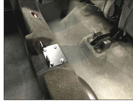
STEP 7 While holding the Bracket in its position, carefully lift the enclosure, then fully tighten the four 3/8 - 16 x 1-1/4" Hex Head Bolts.
