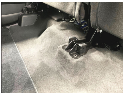
STEP 4 Using an E12 socket and wrench, remove the two inner seat bracket bolts.
