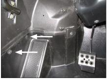
**STEP 2** Remove the two indicated factory bolts.
