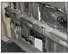
The supplied wax square is to be placed onto the rear wall, just to the right of the second mount as in the picture.
