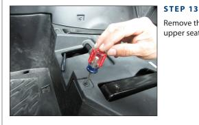
Remove the four clips from the top of the upper seat bracket trim panel.
