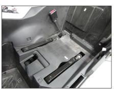
Remove the upper seat bracket from the vehicle.
