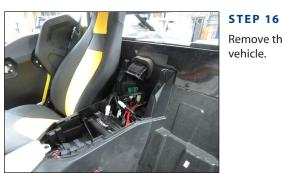
Remove the upper console panel from the vehicle.
