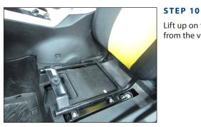
Lift up on the driver's seat, and remove the seat from the vehicle.
