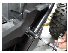
**STEP 9**Remove the seat belt bolt.
