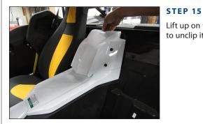
Lift up on the back of the upper console panel to unclip it.
