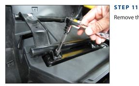
Remove the four upper seat bracket bolts.
