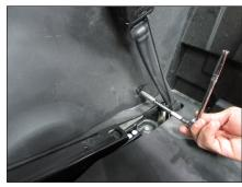
Remove the two clips from the driver's side of the lower console panel.
