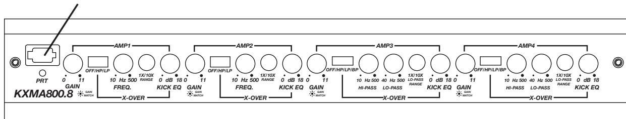
**Automatic Turn-On Selection:** The KXM series offers three different automatic turn-on modes that can be selected on the end panel; +12V, DC Offset, and Audio. Using either the DC Offset or Audio mode causes the REM terminal to have +12V out for turning on additional amplifiers.
