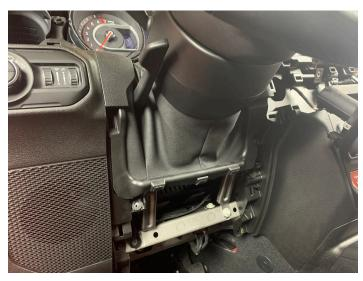
• Install (2) Phillips screws on shroud
