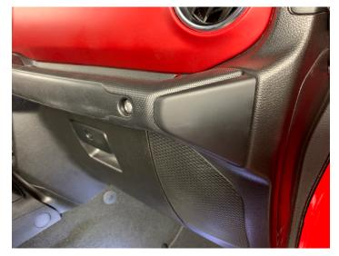
• Install (5) Phillips screws on the side of dash
