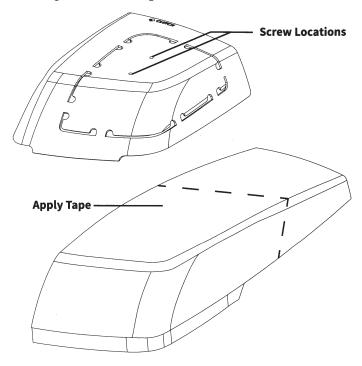
Apply the template to the saddlebag lid and secure using (2) Step 3. screws that came with the kit.
