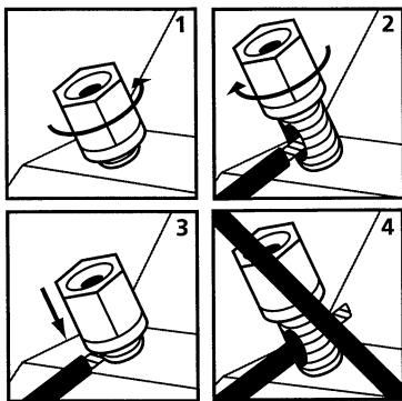
**Using Binding Post connectors.**
