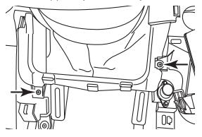
4 Unclip, unplug, and remove the climate control panel.
