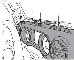
10 Remove panel on the left side of the dash then remove the (5) Phillips screws exposed.
