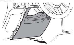
3 Unclip the steering column shroud then set aside.
