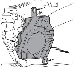
15 There is an electronic module attached to the back of the pod which must be removed and reused in kit assembly.
