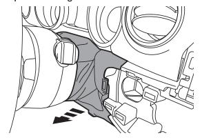
5 Remove the (2) Phillips screws securing the radio trim panel, then unclip and remove.
