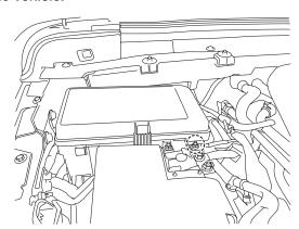
5 Route the Positive (+) power cable through the grommet under the carpet and pull the power cable from under the vehicle. <u>Note:</u> seal the grommet with silicone (not included) to prevent water from entering the cabin.
