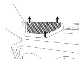
8 Remove (1) Phillips screw securing the dash pad, then unclip and remove.
