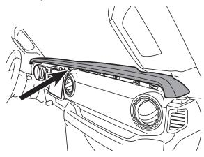
9 Remove the (4) Phillips screws securing the instrument panel on the left side, unclip and remove panel.
