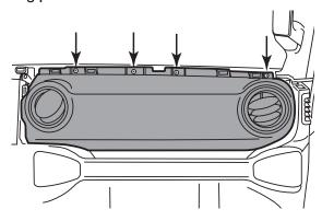
13 Remove the (4) 10mm screws and the (1) 8mm screw securing the dashboard brace. The brace only needs loosened to aid in removing the speaker pod in the next step.
