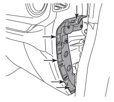
17 Pry outward in the bolt cover on the right end of the grab bar and remove the (2) 10mm bolts securing it to the dash.
