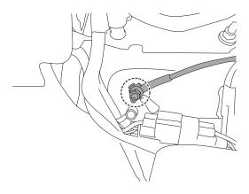
8 Connect the main harness to the amplifier assembly and align it to the seat mounting holes.
