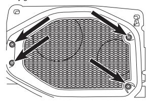
3 Remove gromment holding speaker wire in place and secure speaker wire out of the way.
