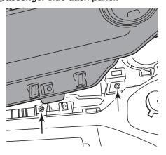
21 Carefully unclip and pull out on the dashboard panel enough to expose the speaker pod. Remove the (3) Phillips, screws securing the pod and remove.
