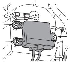
Open the passenger door and remove the panel on the right end of the dash. Remove the (5), Phillips screws exposed.
