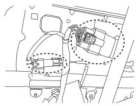
4 Route the power cable following the factory harness along the vehicle's frame and secure using supplied cable ties.
