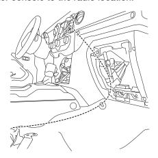
11 Connect the T-harness and the radio with either the Tharness or the RCA adaptors. Refer to page 15 and 16 for the correct system diagram. Return all removed components to their original location.
