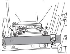
14 Remove the (3) Phillips screws securing the speaker pod, then unplug and remove. the pod.
