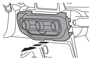
6 Extract the (4) 7mm, screws from the factory radio, disconnect and remove it.
