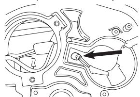
With a reciprocating air saw or preferred cutting device, cut along the line from step 4.
