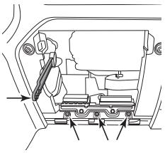
19 Looking up under the airbag assembly, remove the (2) 13mm, bolts that secure the back of the passenger side airbag.
