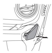
18 Remove the glovebox then remove the (3) Phillips screws exposed.
