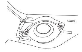
30 Align the factory tweeter grill clips and secure by firmly pressing downward.
