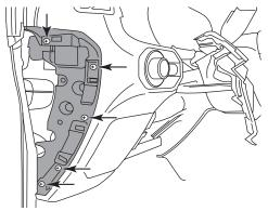
11 Remove the (5) Phillips screws securing the left side dash panel, then unclip and remove.
