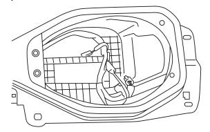
2 Extract the (5) T20, torx, screws from the speakers and the (4) T30, torx, screws from the port and remove.
