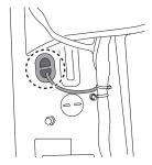
2 Tilt the passenger seat towards the back to reveal (2) connectors, disconnect and remove the seat.
