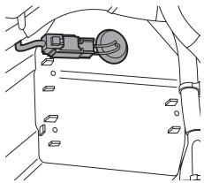
24 Insert the factory wire into the replacement speaker pods and pull gromment thru until it seats into the hole.
