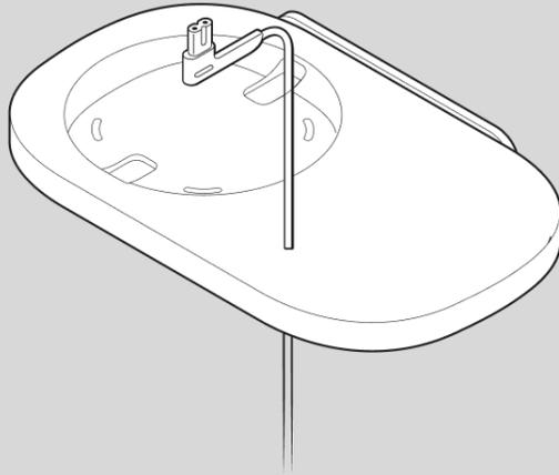
6. Press the bottom cover firmly onto the shelf until it snaps into place, carefully aligning the pins. Plug the power cord into the speaker and place the speaker on top of the shelf.
