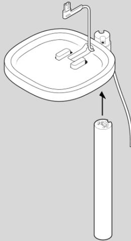
4. Use the 2 silver screws to attach the speaker platform to the top of the stem, threading the power cable carefully. Snap the bottom plate on with the power cable channel in the back, and mount the platform on the stem.
