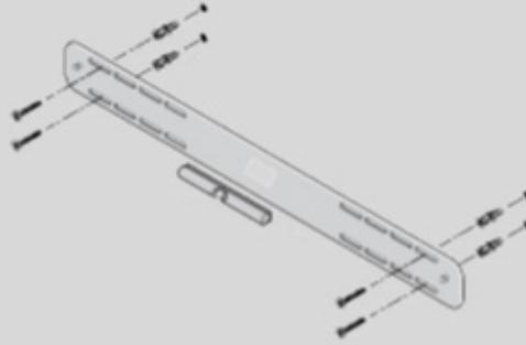
6. Place the bracket on the wall and loosely tighten the screws to secure the bracket. Check with a level and then tighten the screws.
