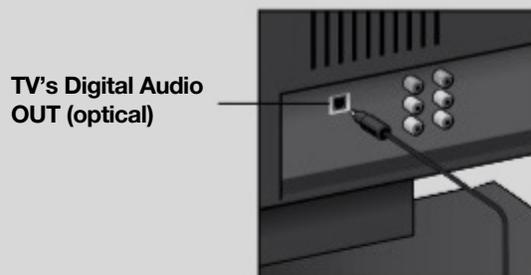
**IMPORTANT:** Remove the protective caps from each end of the optical audio cable before inserting.
