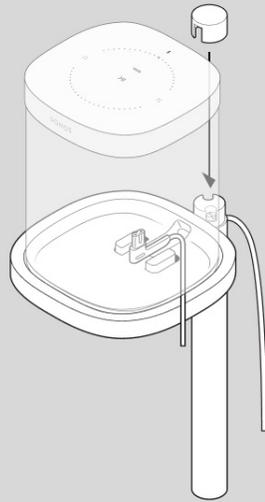
6. Press the power cord into the stem, working from top to bottom. Pull the excess cable down from the base.
