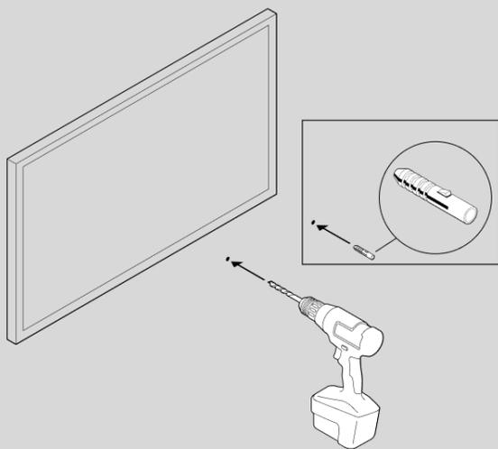
3. If you're using the included wall anchors, use a 5/16" drill bit to drill the pilot holes and then insert the wall anchors. Don't use the anchors if you're drilling into wood or plastic.
