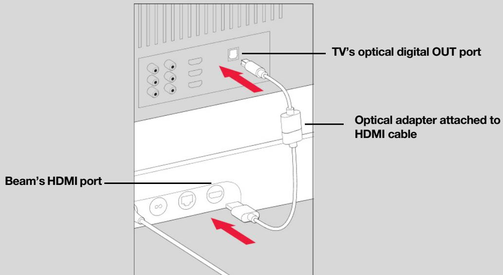
**Note:** The optical adapter's port is "D-shaped"—make sure the connector aligns correctly into the port. Inserting the adapter incorrectly may damage the cable.
