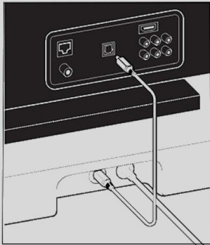
**IMPORTANT:** Remove the protective caps from each end of the optical audio cable.
