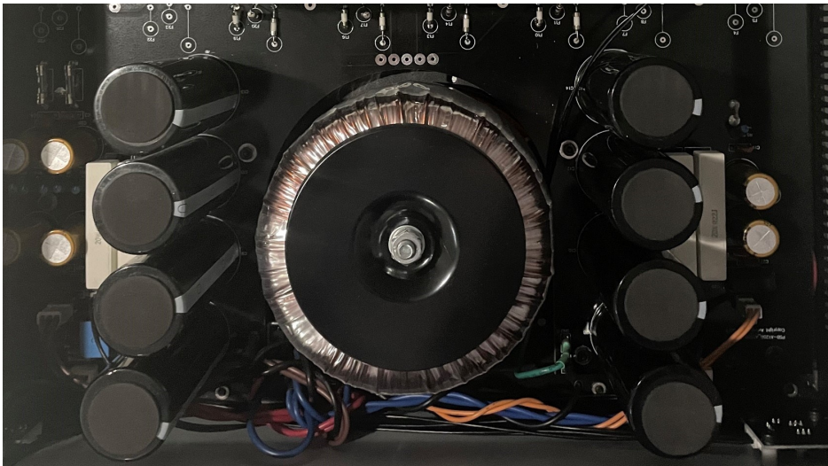
Bryston Class D utilizes massive toroidal transformers with extensive storage capacitance
