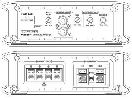
The MX600.1, MX1200.1, MX2000.1, MX3000.1 are equipped with a variable 12db slope Lowpass crossover network and a 12db slope subsonic filter. The mono amps also feature a variable Bass Boost EQ is set at 45Hz. The Bass Boost is helpful in certain subwoofer installations where enclosure location may require an extra boost.
