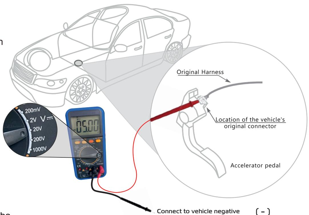
**USE THE MULTIMETER TO CHECK THE END OF THE TIMING OF THE ACCELERATOR PEDAL POWER SUPPLY**
