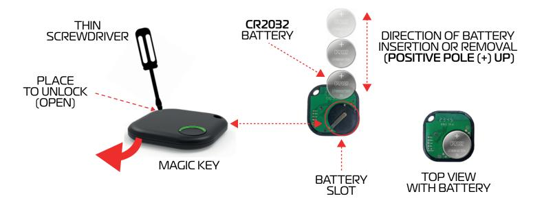
It is possible to monitor when the MagicKey's battery is low and time to be replaced, through the LED signaling of the MagicKey during its activation, where the led will flash twice for 10 seconds, or through the notification automatically generated on the home screen of the FAST MAX app.
