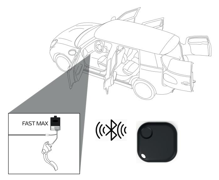
The MagicKey signals its presence to the FAST MAX module via Bluetooth communication, if the MagicKey is out of range of the FAST MAX, the FAST MAX module will initiate progressive lockout of the accelerator pedal to full or partial acceleration Lock, making it impossible to drive, or limiting its driving almost to the maximum while away from the MagicKey.
