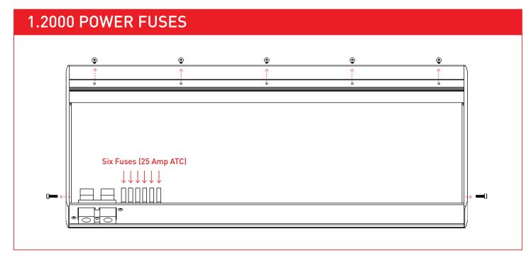
→ TO USE: Remove 5 screws from bottom panel and 2 screws from side panel. 6 x 25 amp ATC fuses
