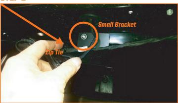
Use the longer screw to mount the <u>smaller</u> bracket to the vehicle. Do not tighten completely until all brackets are threaded into the enclosure. Use the hole on the left to zip tie the harness to the bracket
