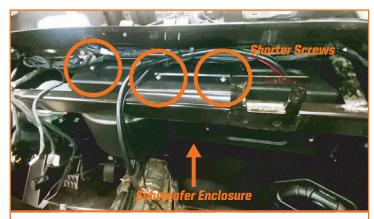
Use the shorter screws to secure the enclosure to both brackets.
