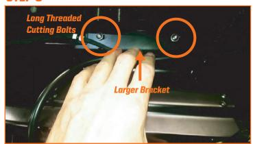
Use the <u>longer thread cutting bolts</u> to mount the <u>larger bracket</u> to the vehicle. Do not tighten completely until all brackets are threaded into the enclosure.
