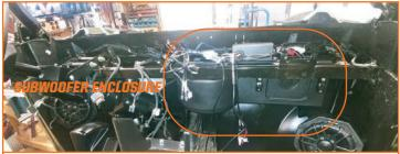
Subwoofer Enclosure Mounting Location, under dash panel in front of passenger seat.
