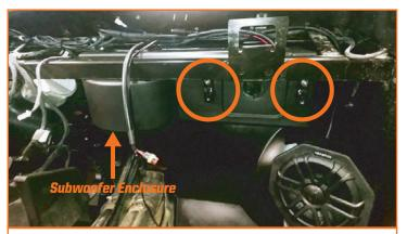
Then secure the <u>lower brackets</u> to the <u>enclosure</u>. Once these are threaded you can proceed to tighten all brackets to the vehicle and subwoofer.
