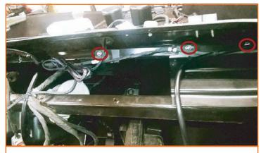
You must de-trim your machine to access the subwoofer mounting location. To do this, remove the vehicle hood, dash trim, front dash assembly and passenger side seat, the grab bar and the center console trim panel and the glove box. You will now have access to the factory bolts to mount your kit. The photo above shows the area you will be working on.
