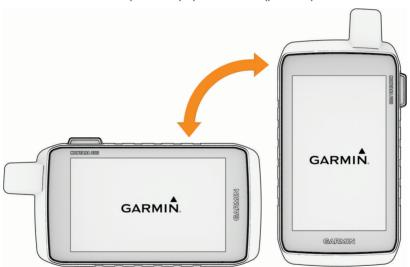
**NOTE:** While using the inReach features of your Montana 700i/710i/750i/760i device, you should use the device in vertical (portrait) mode, with the antenna pointed toward the sky.
