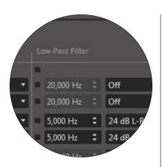
**Passband**: the range of frequencies uniformly passed by a filter. Defined by two frequencies.
