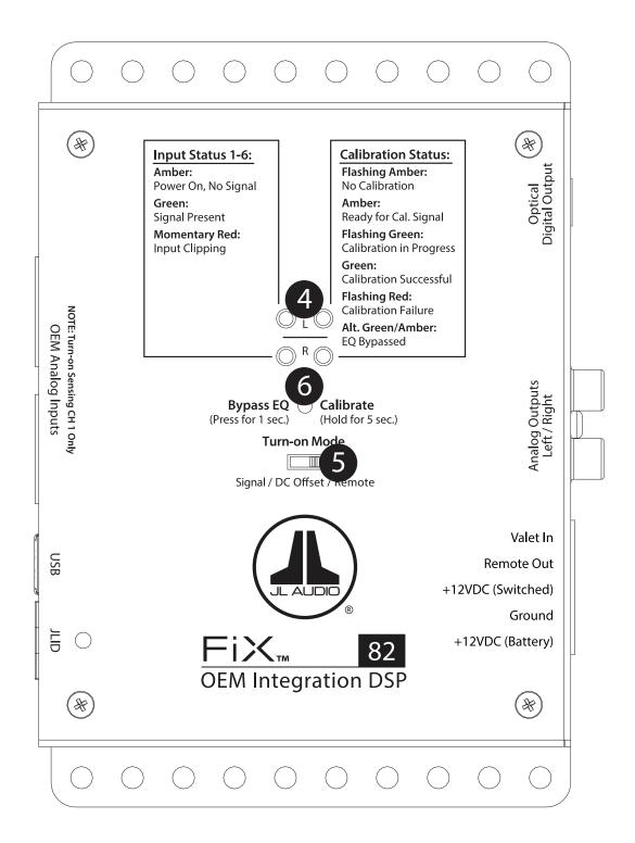
FIX<sup>™</sup> 82 Power Connection / Audio Output Panel
