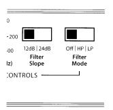
1) "Filter Mode" Control: this switch allows you to configure the filter for that Channel Pair into one of two filter types.
