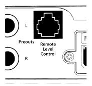
When connected to the amplifier, the HD-RLC operates as follows. At full counter-clockwise rotation, the audio will mute completely. At full clockwise rotation the level will be the same as if the HD-RLC was not connected at all. In other words, it operates strictly as a level attenuator.
