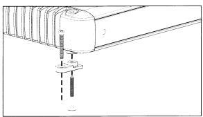
Lateral Mounting Feet are also included with your HD600/4 to provide an alternative mounting option. Each mounting foot should be attached to the bottom of the amplifier by screwing the provided bolt into the bottom of the amplifier and up into the corner cap with the supplied 1/8-inch hex wrench. Next, using appropriate mounting screws (not included), secure the amplifier by its four Lateral Mounting Feet.
