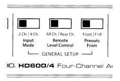
For example, if you are using the HD600/4 in a stand-alone bi-amplified mode, you may want the HD-RLC to only affect the level of the subwoofer channels. Setting the "Remote Level Control" switch to the "Rear Ch." position accomplishes this (provided the subwoofer system is connected to the rear channels).
