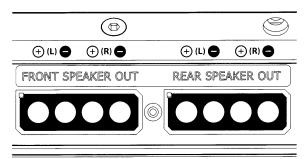
To bridge a pair of channels, use the "Left +" and "Right –" speaker connectors only (the "Left –" and "Right +" remain unused).
