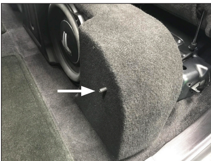
STEP 4 Thread a 3/8 - 16 x 2-1/2" Set Screw into the threaded insert on the bottom of the enclosure, leaving approximately 1/2" exposed. Repeat for the opposite side.
