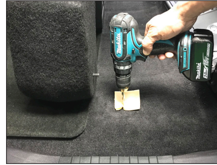
STEP 8 Using a 1/2" drill bit, carefully drill through the impression in the Wax Square. Repeat for the opposite side. Remove the Wax Squares from the vehicle.
