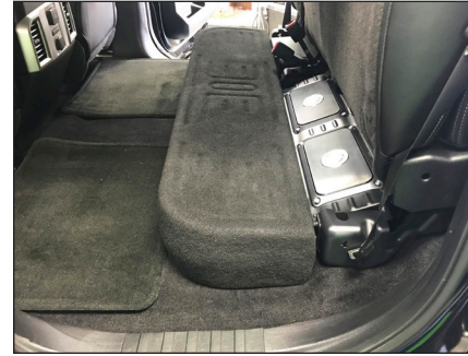
STEP 5 Place the Stealthbox into position, as shown. The enclosure should be centered in the vehicle and pushed rearward until flush against the rear seat bracket bolts.
