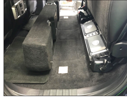
STEP 7 Carefully tilt the enclosure forward, as shown, ensuring the Wax Squares remain affixed to the floor.
