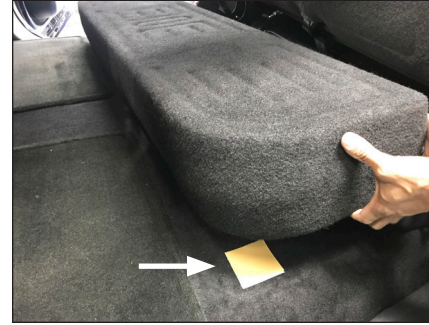
STEP 6 Remove the adhesive from a Wax Square. Lift up on the side of the enclosure, and affix the Wax Square to the floor directly under the 3/8 - 16 x 2-1/2" Set Screw installed in Step 4 . Repeat for the opposite side. Firmly press down on the enclosure so that the 3/8 - 16 x 2-1/2" Set Screws leave an impression in the Wax Squares.
