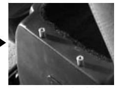
**STEP 27:** Place the pair of supplied aluminum spacers over the two holes that are located at the upper rear of the Stealthbox, From **STEP 11**.
