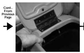
**STEP 28:** Position the OEM console shell over the Stealthbox.
