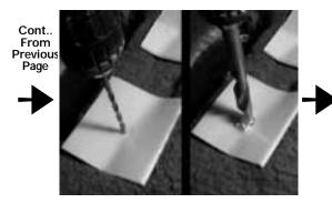
**STEP 18:** With a 1/8" drill bit and drill, drill a pilot hole.
