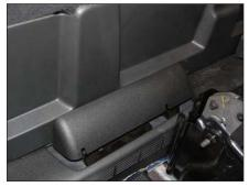
Carefully unclip and remove the two hinge cover panels.
