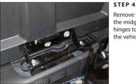
Remove the bolts holding the two hinges to the midgate. Remove the nuts holding the two hinges to the floor. Remove the midgate from the vehicle.
