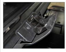
Remove the two latch assemblies from the top of the midgate.
