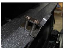
Install each of the factory latches and spacers onto the top of the Stealthbox® using a pair of 1/4 - 20 x 2" Phillips Flat Head Screws.
