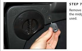
Remove three of the factory rubber stops from the midgate. The factory screws will not be used.
