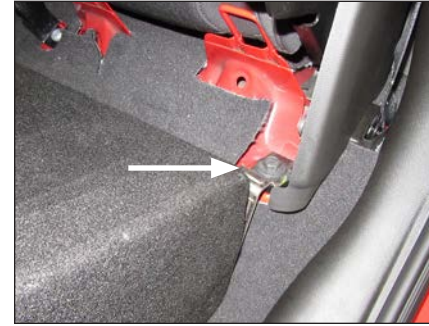
STEP 8 Reinstall the two seat bolts, and hand tighten.
