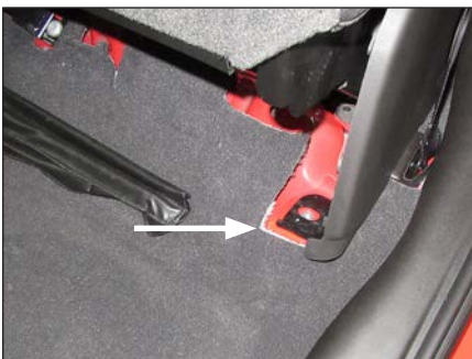
STEP 4 Remove the seat bolt. Repeat for the opposite side.
