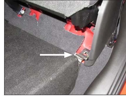
STEP 7 Carefully lower the enclosure into position, allowing each Bracket to fit over the seat bracket. Align the hole in each Bracket with the factory seat bolt hole.
