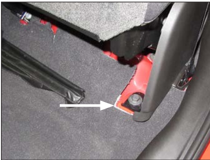
STEP 3 Locate the outer seat bolts.
