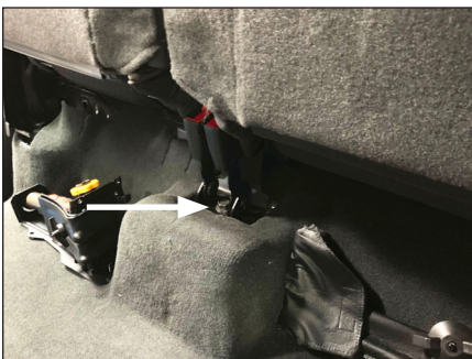
STEP 4 Remove the center seat bolt and seat belt bracket.
