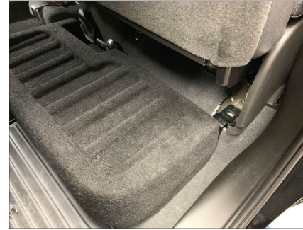
STEP 7 Carefully lower the enclosure into position, allowing the Small Bracket to fit over the outer seat bracket. Align the hole in the Small Bracket with the factory seat bolt hole.
