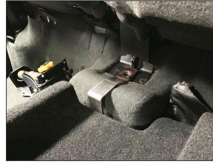
STEP 8 Align the large hole in the Large Bracket with the center factory seat bolt hole. Be sure the alignment pin passes through the small hole in the Large Bracket.
