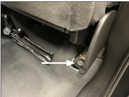
STEP 3 Remove the outer seat bolt on the driver's side.
