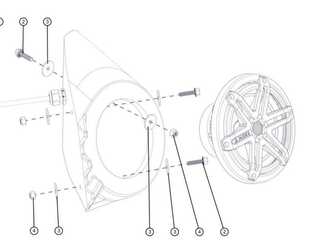
Note: For optimum performance, JL Audio recommends applying the included Foam Strips (or sound damping material) to surrounding plastic panels to reduce unwanted vibrations.
