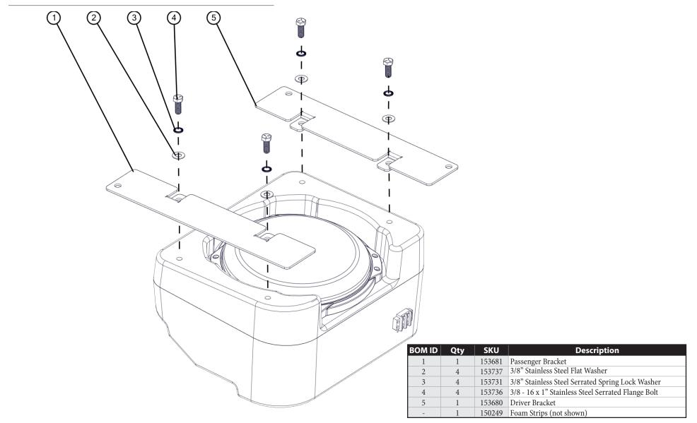
Note: For optimum performance, JL Audio recommends applying the included Foam Strips (or sound damping material) to surrounding plastic panels to reduce unwanted vibrations.
