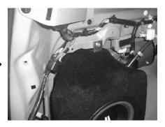
**STEP 15:** Place the Stealthbox in its proper location, making sure to place the threaded rod into the previously drilled hole in the floor.
