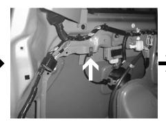
**STEP 12:** Insert the supplied U-bolt in factory hole.
