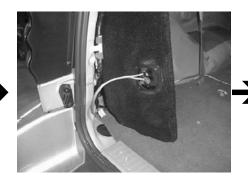
**STEP 13:** Run speaker wires to the location of the Stealthbox. Check the Stealthbox for proper operation.
