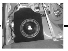
**STEP 17:** Fully tighten the bolt on the top of the enclosure and the nut on the threaded rod on the bottom of the enclosure to secure the enclosure.
