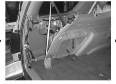
STEP 2: Remove the driver's side rear panel.
