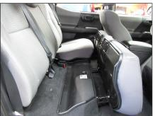
**STEP 2** Fold the passenger side seat bottom forward.
