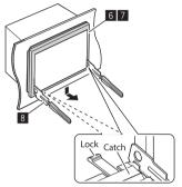
2 When the lower level is removed, remove from the upper two catches of the trim plate (5/7).
