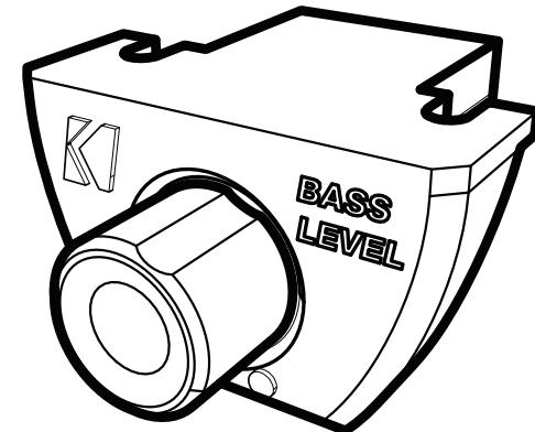
With the CXARC remote bass level control, you have the ability to attenuate the output level of the amplifier remotely. To surface-mount the CXARC remote bass level control, simply screw the remote to the chosen location, then run the cable from the controller to the "Remote Bass" jack on the amplifier panel. Do **NOT** connect/disconnect while the amplifier is on. Connecting the 3.5mm cable without the remote knob will cause the amplifier to output at full gain, possibly damaging your speakers.
