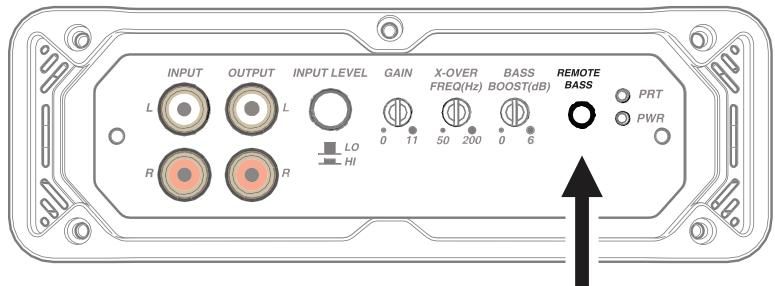
Remote cable passes audio; do not run cable parallel to power wires.
