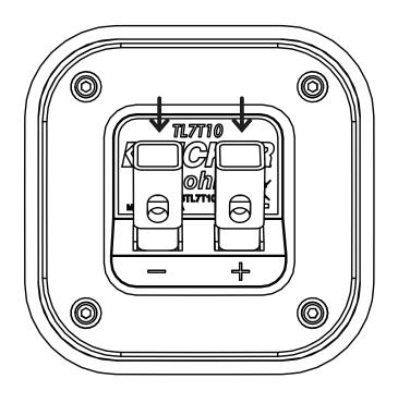
**Sound Check:** Poor bass response? Check the system phasing by reversing the positive and negative speaker connections on the subwoofer. If the bass improves, then the subwoofer was out of phase in reference to the rest of the audio system.
