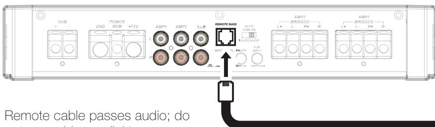
Remote cable passes audio; do not run cable parallel to power wires.
