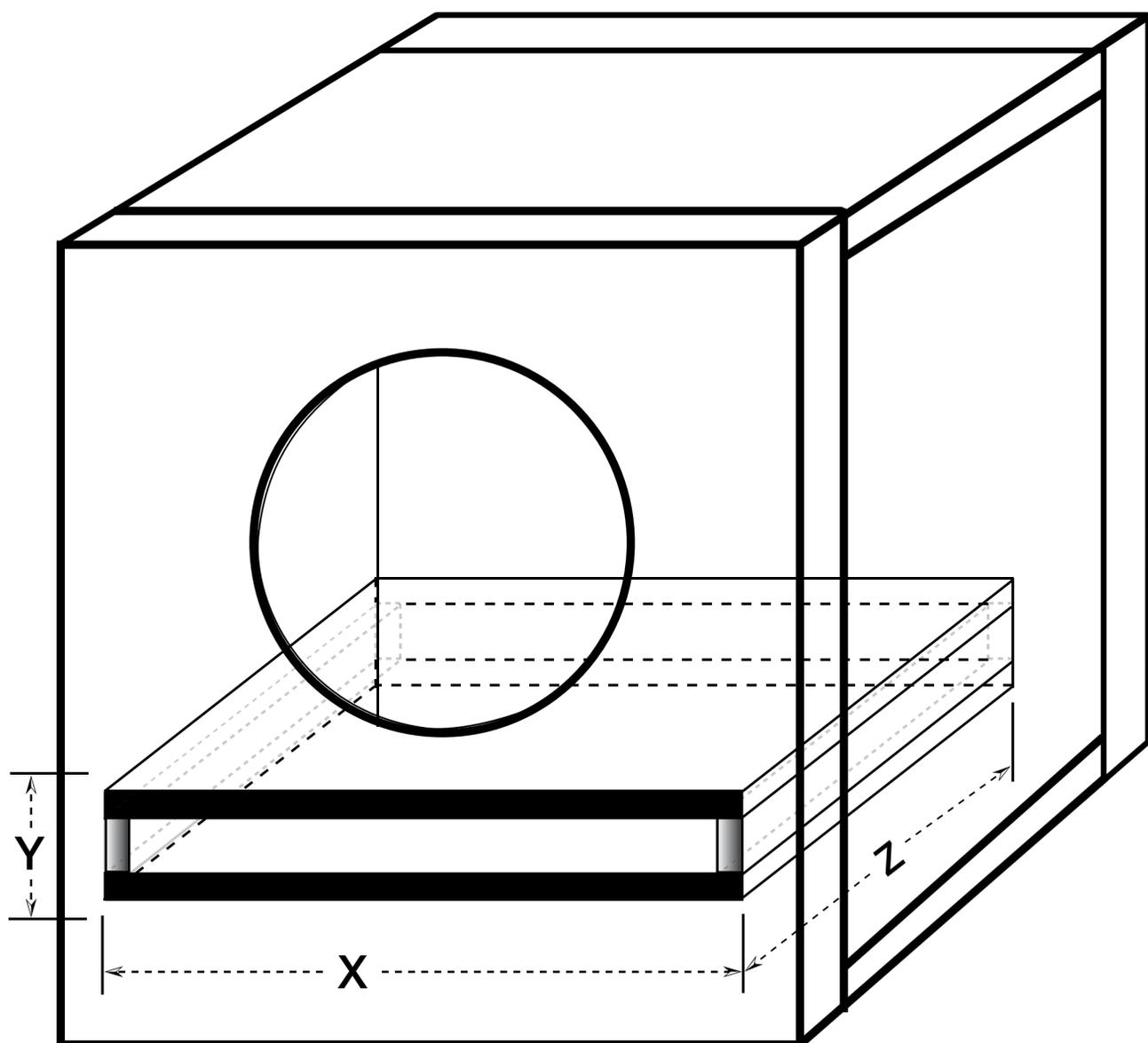
You can loosely fill your enclosure with poly-fil stuffing. Ported designs will require covering the end of the port (located inside the box) with grill cloth, chicken wire, or expanded metal to prevent the poly-fil from exiting the port. The use of poly-fil will slightly decrease efficiency, but will deepen and extend the low frequency output by making your subwoofer think it's in a bigger box.
