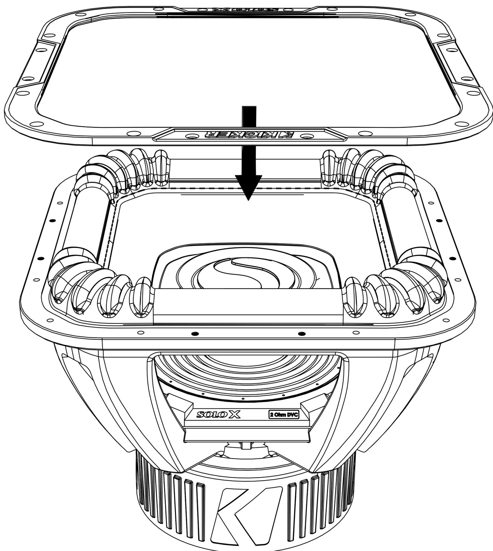
Secure the Surround Mounting Flange to the basket with the eight M5x0.8x10mm bolts. Loosely start all bolts before tightening. Torque bolts to 20in-lbs in the sequence shown below.
