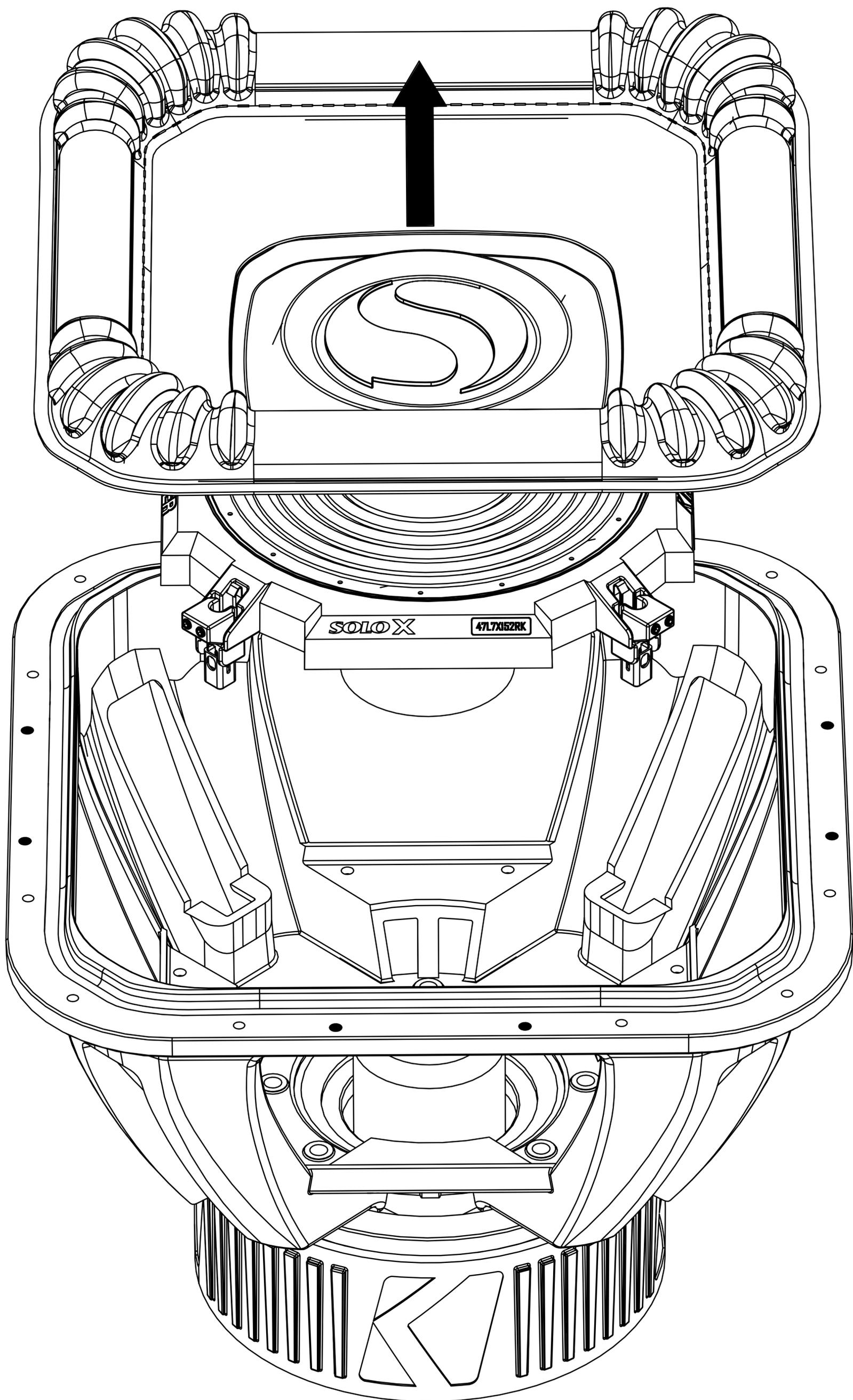
Clean and remove all debris from the Voice Coil Gap.
