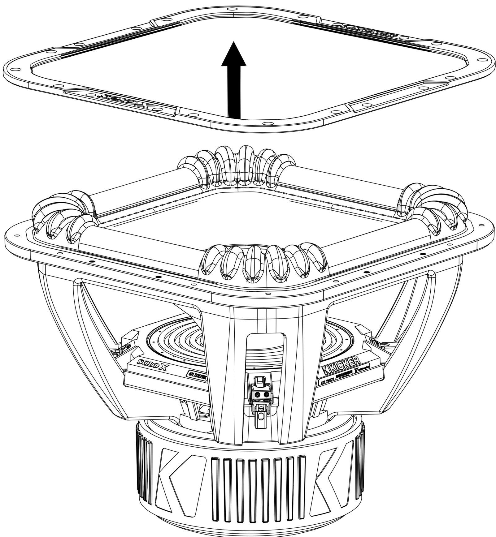
From the magnet side (bottom) of the Basket Assembly, use a 4mm Allen Wrench to remove the eight M5x0.8x16mm bolts securing the Spider to the Basket Assembly.
