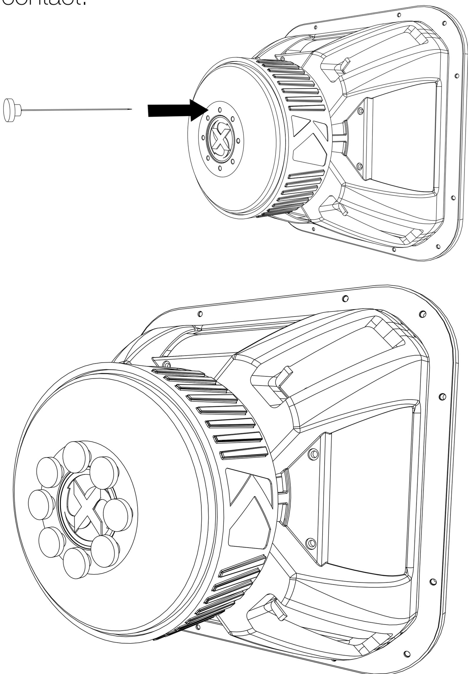
After all the Voice Coil Alignment Pins are inserted, push the pins towards the magnetic pole until the pins are held to the pole magnetically. Space the pins evenly around the pole.
