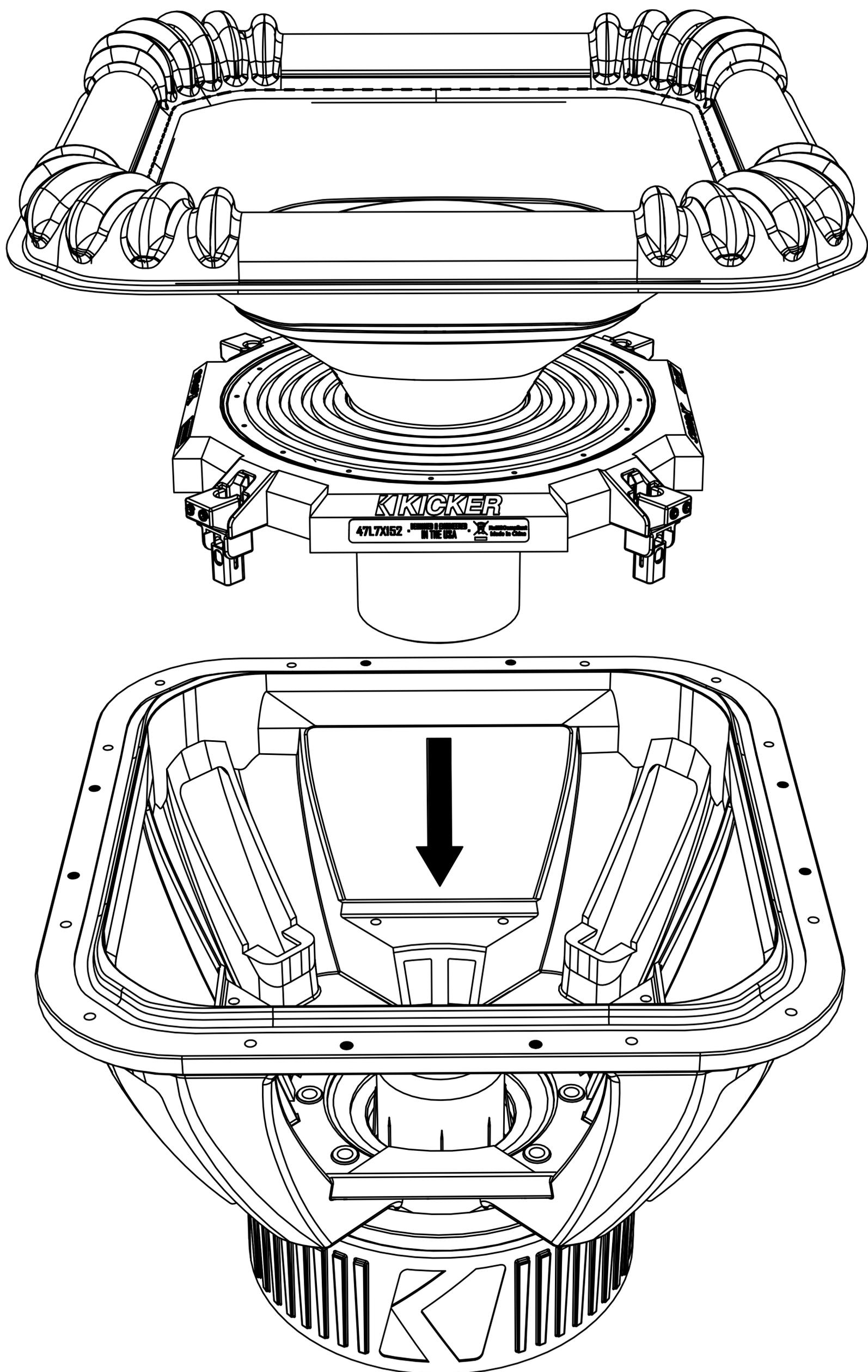
Secure the Spider to the Basket Assembly using the eight M5x0.8x16mm bolts. Loosely start all bolts before tightening. Torque the bolts to 20in-lbs in the sequence shown below.
