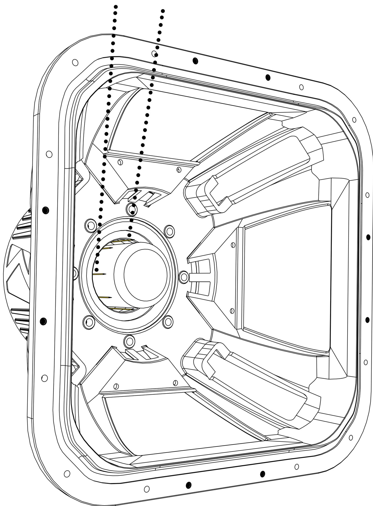
With the Basket Assembly still laying on its side, insert the new Cone Assembly into the Basket Assembly. Pay close attention and ensure that the pins lay inside of the voice coil, allowing the voice coil to smoothly slide into place over the magnetic pole.
