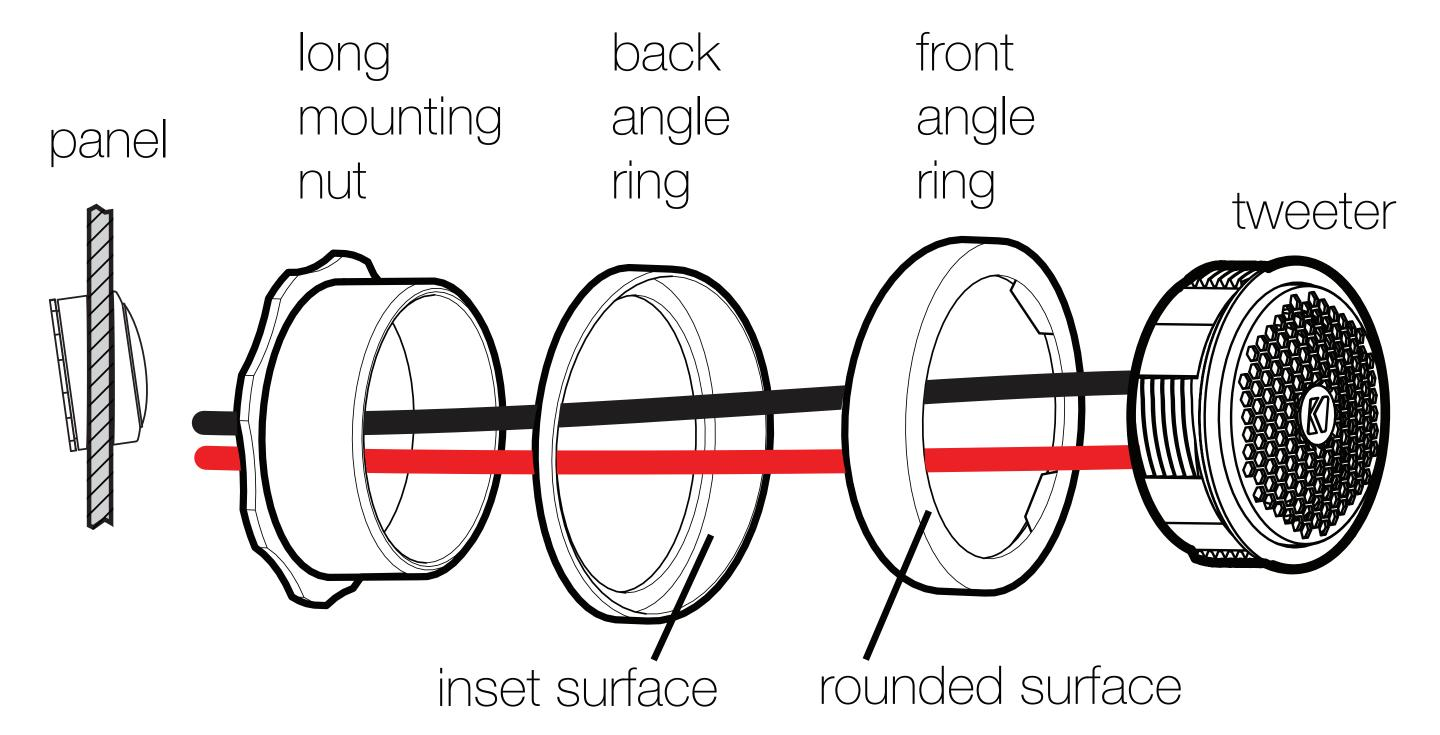
Use a 1/8 turn with tweeter tool to secure the tweeter to the mounting nut.
