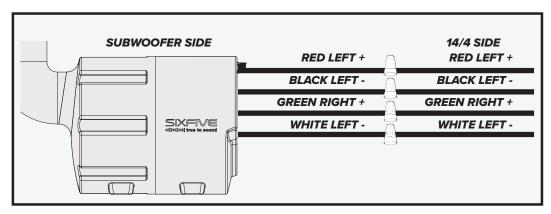
The subwoofer can be place anywhere in the line. You will need to continue the 14/4 wire out of th wire nut to the next speaker in line staying consistent to the original wire pattern you started prior to connecting your subwoofer. The subwoofer wires are color coded to match standard 14/4 wire.
