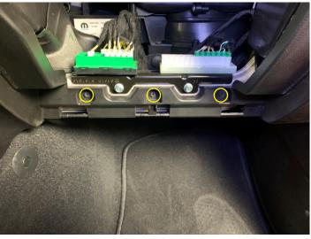
• Looking in the glovebox cavity up high, remove two 13mm bolts securing the back of the passenger side airbag
