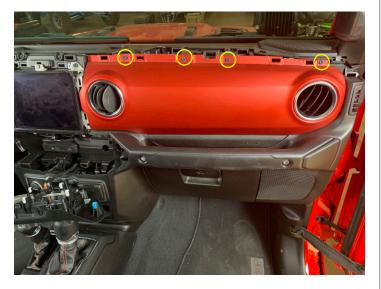
• Unclip and remove the panel on the side of the dash
