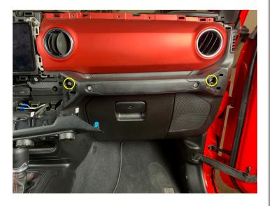
• Slide ears on cover into slot and snap grab handle cover into place
