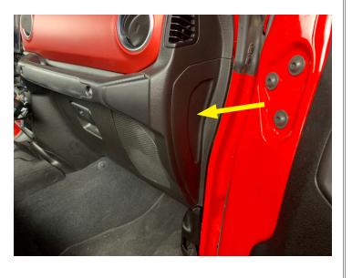
• Install (4) Phillips screws on the top of the air bag
