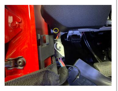
• Remove (2) Phillips screws near steering column
