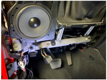
• Install (4) 10mm bolts below steering column. (one is hidden behind the cross brace behind the left down support)
