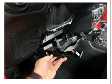
• If you are replacing the top dash speakers, make sure to connect the wires that you passed from the lower pod to the speaker
