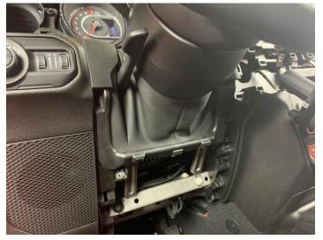
• Install (2) Phillips screws on shroud
