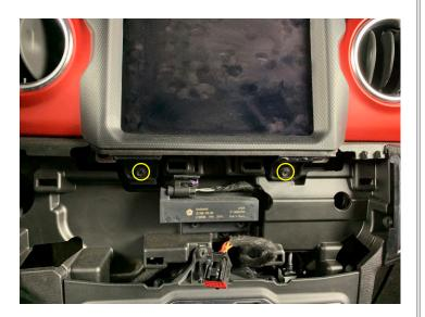
• Remove (1) Phillips screw securing the front dash pad, carefully unclip and remove by pulling forward toward the front seats
