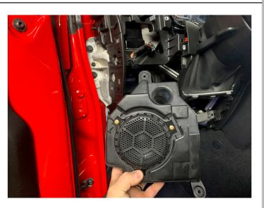
• Remove the module from the OEM enclosure
