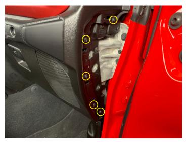
• Using a panel tool carefully remove the grab handle cover (starting on the left)
