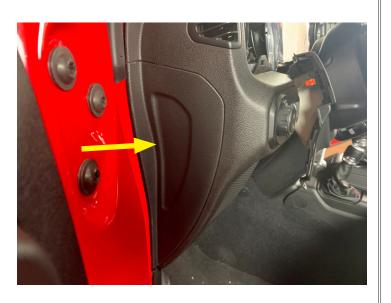
• Clip the steering column shroud into place
