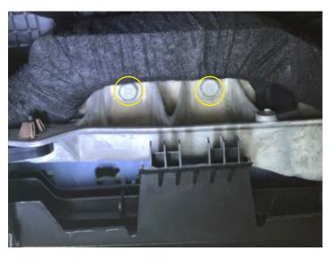
• Carefully unclip the air bag. (this does NOT need to be removed from the vehicle)
