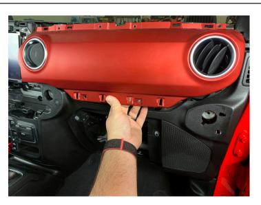
• Lifting the airbag slightly will expose (5) Phillips screws that need to be removed
