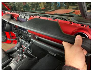
• Carefully unclip the instrument panel shroud along the bottom and remove
