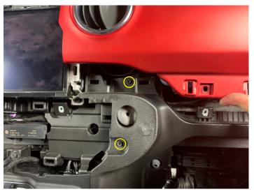
• Remove (3) Phillips screws holding the passenger speaker enclosure, then disconnect wires and remove from vehicle
