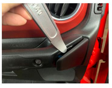
• Remove (2) 10mm bolts securing the grab handle and set handle aside
