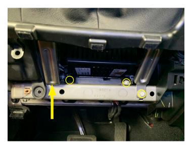
• Remove (1) 8mm bolt below the speaker and this will free the lower support brace to aid in the removal of the speaker enclosure
