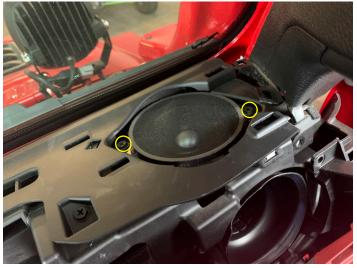
• Install new speaker enclosure and secure with (3) Phillips screws
