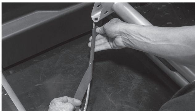
Step 7 - Wrap the brake line with the strip of adhesive backed foam tape included in the box. Note: This step is to prevent the brake line from rattling against the enclosure under high bass output and any chaffing due to movement of the brake line while the vehicle is in motion.
