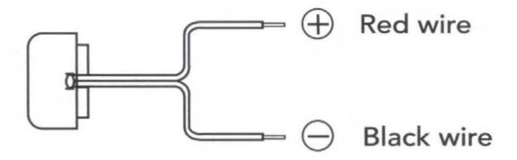
The Red & Black Wires are to be connected to the corresponding outputs of a source unit or power amplifier.
