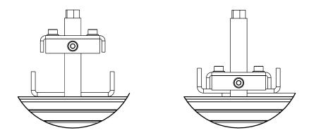
With the Sliding Rails positioned as far down as they can go, please tighten the shaft screw (L) on each of the four Sliding Rails.
