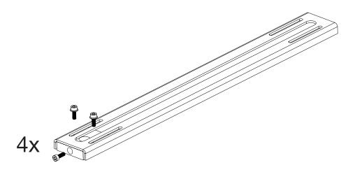
Position each of the four Sliding Rail assemblies over the Fixed Rails (and their spacers), with the bracket side pointed downwards.
