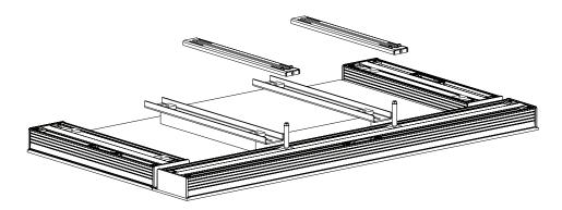
Slide the assembled Sliding Rails over the Threaded Shaft. The Sliding Rails should have one end through the Threaded Shaft and the other resting on the Static Rails.
