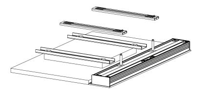
Slide the assembled Sliding Rails over the Threaded Shaft. The Sliding Rails should have one end through the Threaded Shaft and the other resting on the Static Rails.
