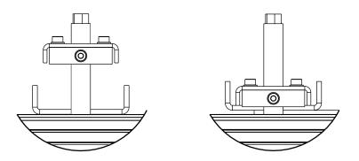
Please tighten the threaded shafts and their corresponding screws on the sliding brackets.
