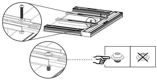
With your horizontal soundbar (1C/1S/1SC) mounting almost complete, begin the installation of your two vertical soundbars (2S/2SC). Start with the Fixed Rails (QTY 4x).
