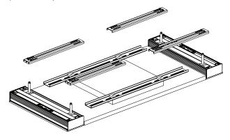
Slide the assembled Sliding Rails over the Threaded Shaft. The Sliding Rails should have one end through the Threaded Shaft and the other resting on the Static Rails.
