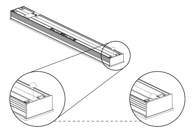
Screw the Wall Mount Bracket onto the wall using screws (not supplied). Seek professional advice for the appropriate screw hardware for your wall construction. Depending on the weight of your soundbar and the construction of walls, it is highly recommended you screw into wall studs.
