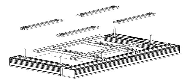
Slide the assembled Sliding Rails over the Threaded Shaft. The Sliding Rails should have one end through the Threaded Shaft and the other resting on the Static Rails.
