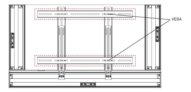
Please position the Fixed Rails (QTY 2x) over the previously installed rail set and ensure alignment over the TV's VESA inserts. Please use the provided VESA screws to maintain alignment throughout the remainder of the installation process.
