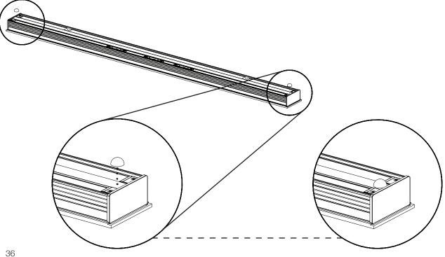
Ensuring the Wall Mount Brackets are level, attach them to the wall using screws (not supplied). Seek professional advice for the appropriate screw hardware for your wall construction. Depending on the weight of your soundbar and the construction of walls, it is highly recommended you screw into wall studs.
