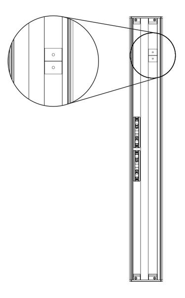
Attach the Extrusion Side Bracket to the Extrusion Brackets using the included Flanged Screws.
