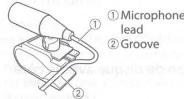
**2 Install the microphone clip on the sun visor.**
