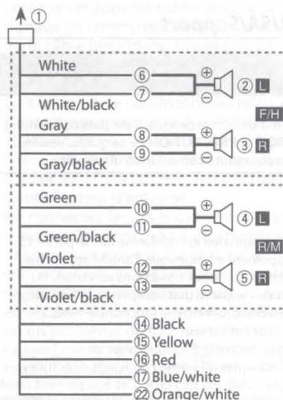
Perform these connections when using a subwoofer without the optional amplifier.
