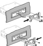
4 Detach the monitor cable cover from the LCD screen (3), then connect the monitor cable to the LCD screen (3). After that, attach the LCD screen with adjusting the up-down position (3) to this unit by using the screws each side (3).
