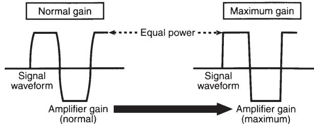
If the signal waveform is distorted due to high output, even if the amplifier gain is raised, the output power will change only slightly. □
