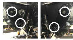
2. Remove four inner fairing bolts using a T25 Torx driver. Two inner fairing bolts are located below each glove box, adjacent to each wind deflector. Store these screws in a safe place for installation later.
