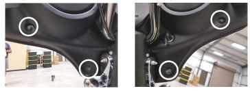
3. While straddling the front wheel fender, grasp the outer fairing, remove the center outer fairing bolt from the previous step, then gently pull the fairing apart from the bike. With the fairing slightly pulled away from the bike, disconnect wire harness for the headlamp and any other accessories. Lay the fairing on a protected flat surface to prevent damage.
