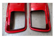
5. Following the traced cut-out lines, cut away the speaker opening from each lid. If using a jig-saw or air-saw, pre-drill a 3/8" hole within the cut-out area to accomodate the start of your cut. After the center section has been cut away, use a metal file to smooth-out any rough edges and corners. SAFETY GLASSES ARE A MUST!!!!
