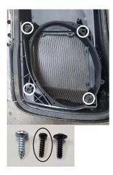
6. While holding the grill in place on the top surface of the lid, turn the lid over and line-up the speaker adapter screw holes. Use four small headed phillips screws provided to attach the speaker adpater to the grill.
