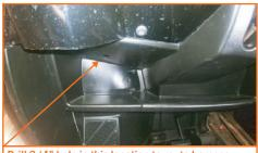
Drill 3/4" hole in this location to route harness though.
