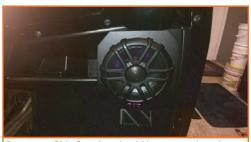
Passenger Side Speaker should be mounted as shown above and securely tightened.
