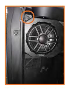
Place the speaker pod into position and secure the factory T25 and T40 torx screws through the brackets attached to the speaker pod.
