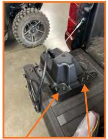
Using the supplied M6 screws and small washers, install the supplied brackets to the speaker pods
