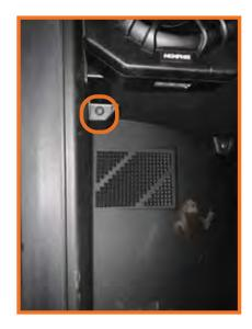
Remove the factory T25 torx screw located underneath the dash
