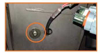
From the top side of the dash, secure the M6 top mounting screw and large washer to the pod though the smaller hole next to the routed speaker wire
