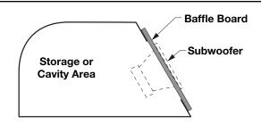
**NOTE:** When using vented enclosures, for maximum reliability and power handling ensure, that a subsonic or "infrasonic" filter is used so that only usable low frequency signal is sent to the subwoofer.
