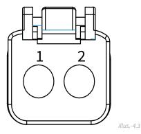
Speaker Pin Out (wire side) 1 - RED - Positive Speaker Input 2 - BLACK - Negative Speaker Input **NOT included with speakers** Connector is DEUTSCH<sup>TM</sup>/Amphenol style DT06-2S
