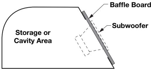
An Infinite Baffle enclosure design represents an application where the compliance of the air volume within the enclosure is greater than the compliance on the speaker's suspension ( $V_{as}$ ). An infrasonic filter is required for reliable performance.
